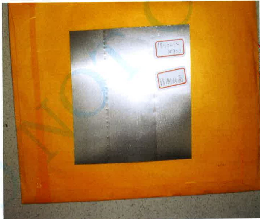
Material: Cell Phone case/Tablet/Laptop bag sleeve Anti Radiation Materials(X-Metal MX-FKR120) Length:120mm, Width:120mm.
